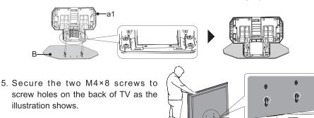
6. Hang the assembled Part a1 and Part B to the two M4×8 screws you have secured to the TV, then secure the assembled part to TV with four M5×16 screws. You can adjust the height of base stand to H1 or H2. For H1, secure screws to four hole 1. For H2, secure screws to four hole 2.
