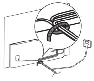
Attach the three covers when installing the wall mount. (Only when the item is provided.) (Only OLED55/65E9\*)
