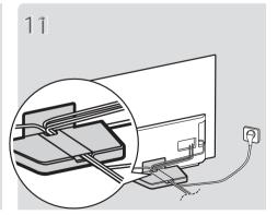
When attaching the stand to the TV set, place the screen facing down on a cushioned table or flat surface to protect the screen from scratches.
