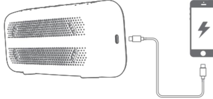
Use the speaker's USB-C port to connect and charge external devices.
