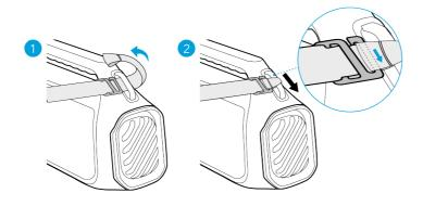
• Attach the strap to both sides of the handle.
